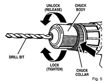
WARNING: Do not hold chuck body with one hand and use power of the drill to tighten chuck jaws on drill bits. Chuck body could slip in your hand or your hand could slip and come in contact with rotating drill bit. This could cause an accident resulting in serious personal injury.
